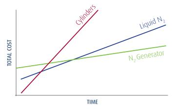
The payback period can be less than one year, when compared to cylinder supply and two to three years, when compared to liquid nitrogen supply.
