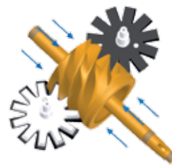
Axial loads act on both sides of the main rotor.
